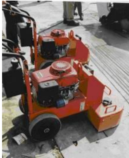
Floor Grinders can be used to quickly fix high spots on a variety surfaces.
