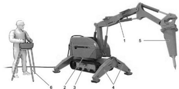
Although the operator is controlling the robot by remote control and not physically in or on the machine, they are still in the work zone, thus are required to use the proper personal protective equipment (PPE) when operating the robot. At a minimum the operator should use:
