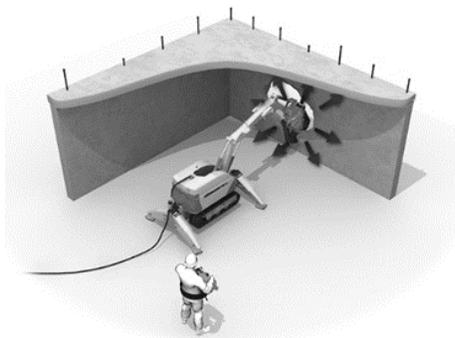
**4.2 Short walls with vaults when using crushers:**
